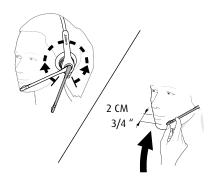
Jabra Biz 1500 has a 270° boom arm so it can be easily adjusted without breaking.
