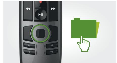
The device comes with a touch sensor. This allows the user to easily control and navigate within applications while recording, without having to switch between the mouse and microphone.
